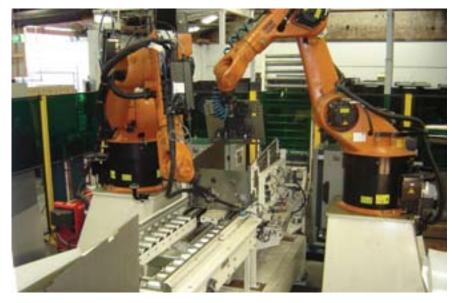
The new Automated Cabinet Welding Line was designed and installed (i) to address occupational health and safety issues by reducing manual handling risks, (ii) to improve welding consistency and quality and (iii) to reduce costs. The Automated Cabinet Welding Line completes the automation of the cabinet manufacture process. It was commissioned during the second half of 2005.
